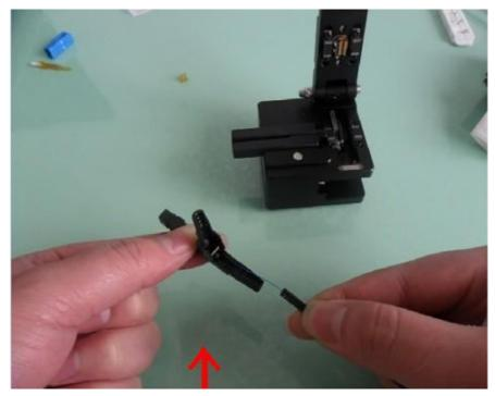
Insert the fiber to the top of the pre-embedded fiber, the fiber will be bending if
