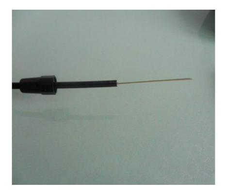
5,use coat stripper to strip the coat 25mm,use cleaning tissue and alcohol to clean the bare fiber.250U fiber length should be 40mm.
