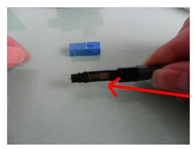
Push down this button and pull out the fiber and repeat installation steps.
