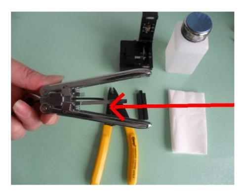
3,use jacket removing tool to remove the jacket
