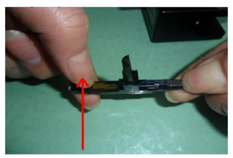
Keep fiber slightly bending position, then push up this button to fix and lock the fiber.
