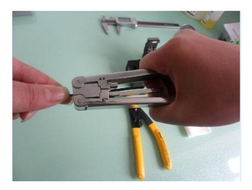
4,check the 250U fiber if it is damaged.flick the fiber with your finger to check if it is complete.
