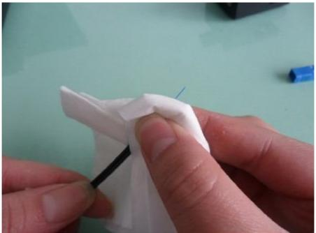
6,fix the bare fiber and use cleaver to cut the bare fiber(take care if the fiber end can be cutted).
