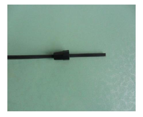
2,fix the cable to length 35mm and strip the jacket
