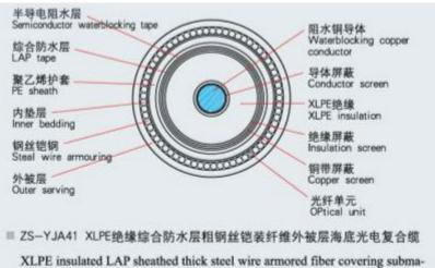
XLPE insulated LAP sheathed thick steel wire armored fiber covering submarine Optical fiber composite power cable
